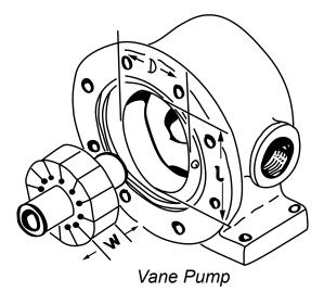
When replacing a pump, catalog ratings will usually be shown in GPM at a specified shaft speed. On motors, catalog ratings will usually be shown as CIR (cubic inches displacement per shaft revolution). Formula are shown for calculating either GPM at 1800 RPM or calculating CIR. Use the formula which is appropriate.
